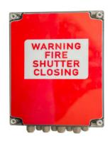
A popular extra for fire shutters is an audio-visual panel which provides a warning that the fire shutter is about to close automatically via the fire alarm system. The panel requires a 240 volt supply together with an appropriate signal from the fire alarm system. The panel also includes a battery backup system and an adjustable timer close facility.
